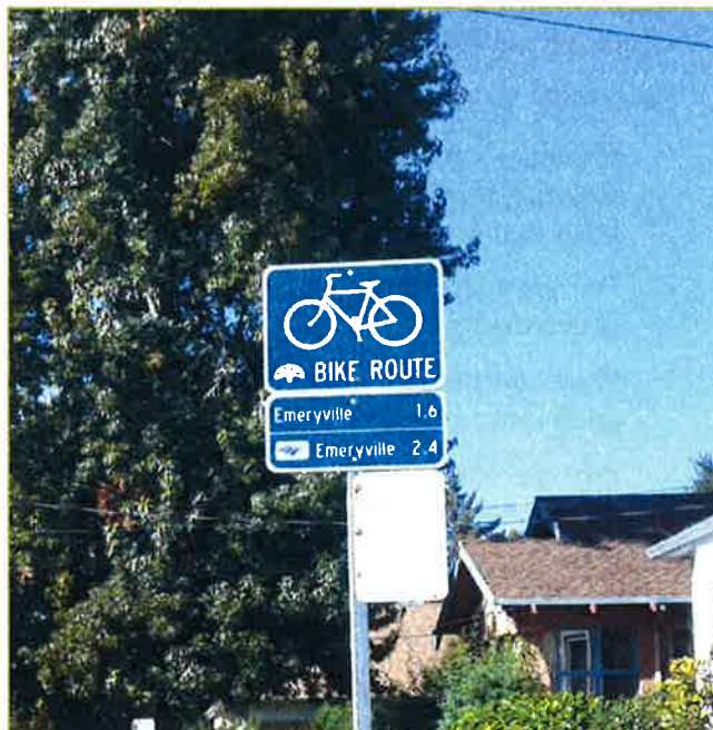
FIGURE 7.3. BICYCLE ROUTE AND GUIDE SIGNS
